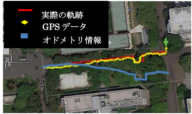
Fig.3. Trajectories of the robot obtained by the GPS and the odometry
