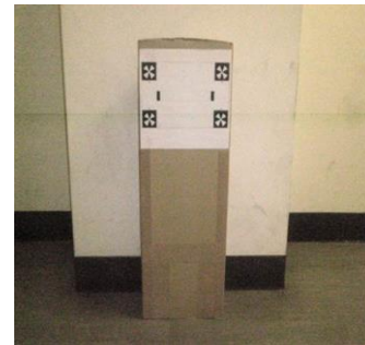
Fig.3 . Guidepost involving artificial landmark (4 marks on the corners) for localization and a barcord at the center for indicating the direction to go.
